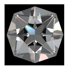
A modification of Gem2 to demonstrate the affects of changing outline by changing girdle index spacing from 4 to 5. Unaltered angles produced a big head shadow and loss of brightness. Raising the crown and pavilion angles corrected this.
